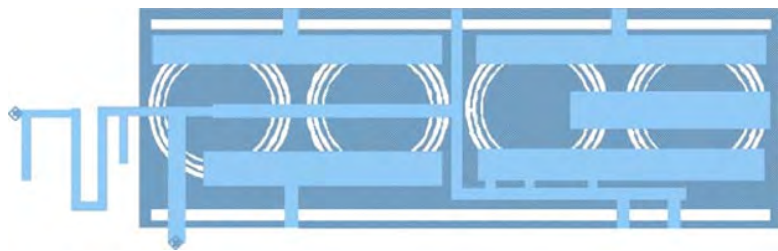
FIGURE 12.16 Wideband antenna with SRR and metallic strips.
