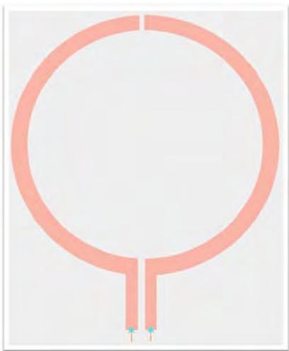
FIGURE 13.14 Loop antenna with ground plane printed on 0.4 mm thick substrate.
